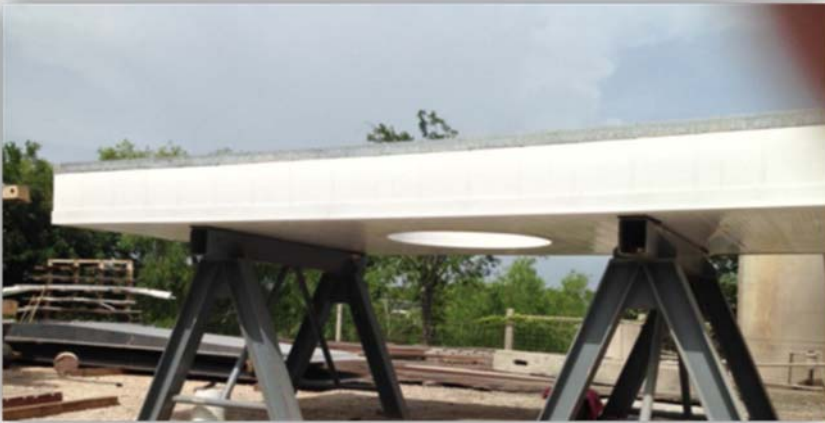
10'x16' Precast Concrete Structure Lid using Danby PL3E PVC liner (2 lids sections)
