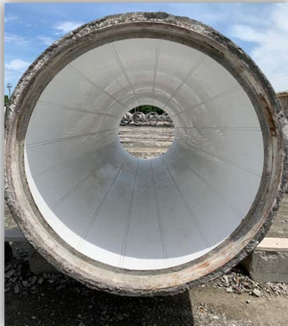
60"x20' PCCP pipe lined with Danby PL3F PVC liner
