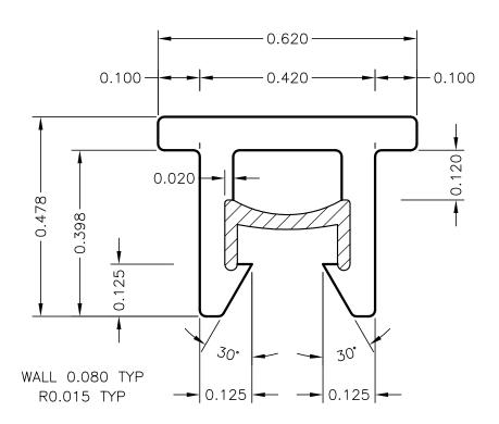
Weight: 0.081 lbs/ft Hatched Area Is Thermoplastic Elastomer
